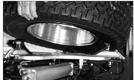
Figure 31B - Outside Clamped with Tire Removed
