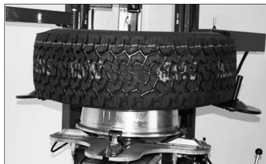
Figure 12 - Lift the Tire for Lower Bead Removal
