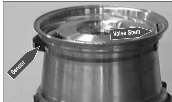
Figure 25 - Wheel with Strapped on Low Pressure Sensor/Transmitter
