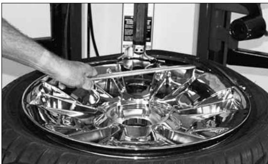
Figure 35 - Start Upper Bead Removal
