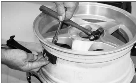
Figure 24 - Rim with a Valve Type Sensor (Tire Removed for Clarity)
