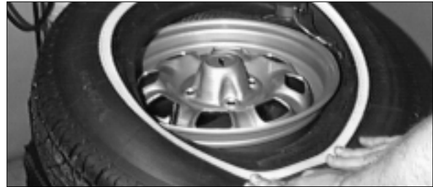
Figure 17 - Mounting Top Bead
