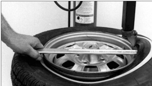
Figure 11 - Lift Bead Over Demount Head
