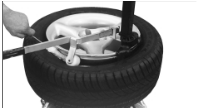
Figure 26 - Lubricate Upper Bead
