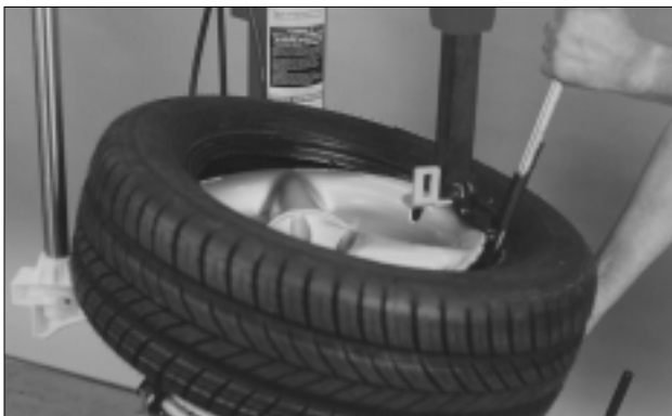
Figure 32 - Helper Holding the Lower Bead in Drop Center
