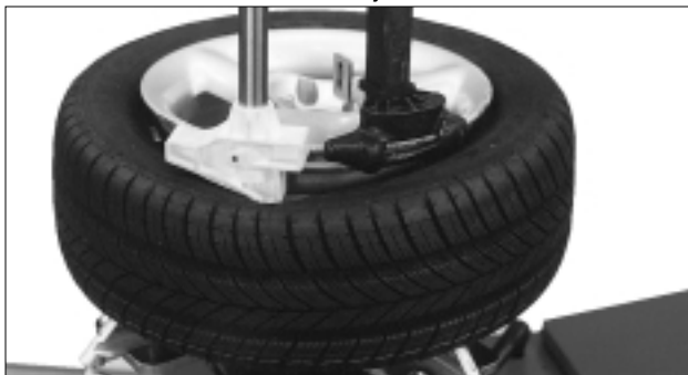
Figure 25 - Helper Foot Depressing Sidewall of Tire
