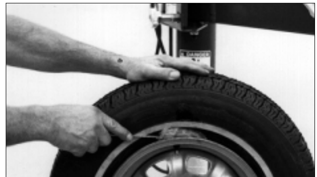
Figure 3 – Apply Rubber Lubricant to Tire Beads
