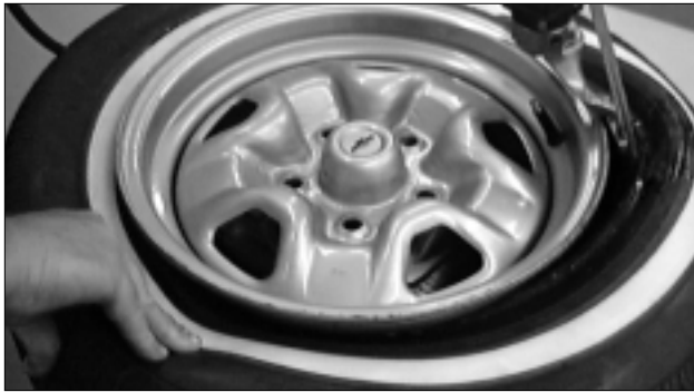
Figure 10 - Insert Bead Lifting Tool
