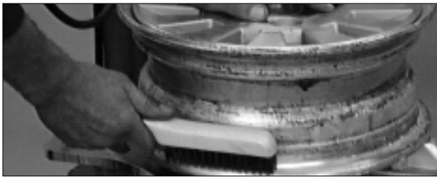
Figure 14 - Inspect and Clean the Wheel
