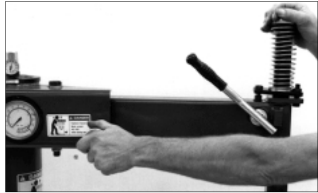
Figure 7 - Adjust Swing Arm to Position Head Roller
